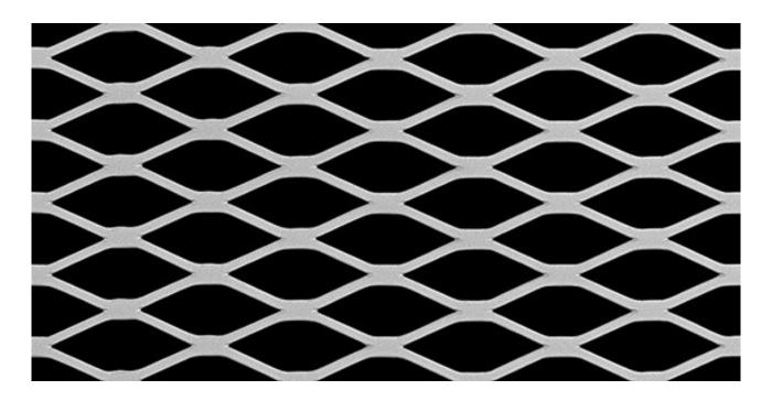
LW Aperture:33.53mmStrand Width:2.31mmSW Aperture:12.45mmThickness:1.20mmWeight:2.47 kg / m2Open Area:73%
